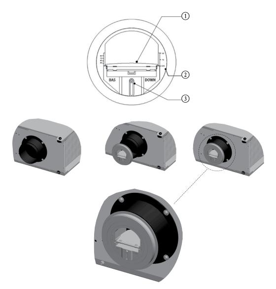
NOTE: To ensure the flow rate controllers operate correctly, a differential pressure of between 60 and 210 Pa is required.
