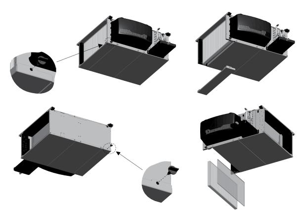
Size 5 also has a hatch, but it is attached in a different way, as shown below.
