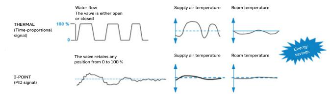
A 3-point motor actuator enables a valve to be actuated as close as possible to the control system requirements, by controlling its position between 0 and 100 % (water flow control). The terminal unit supply air temperature is more stable and the room temperature varies very little (variations cause discomfort).
