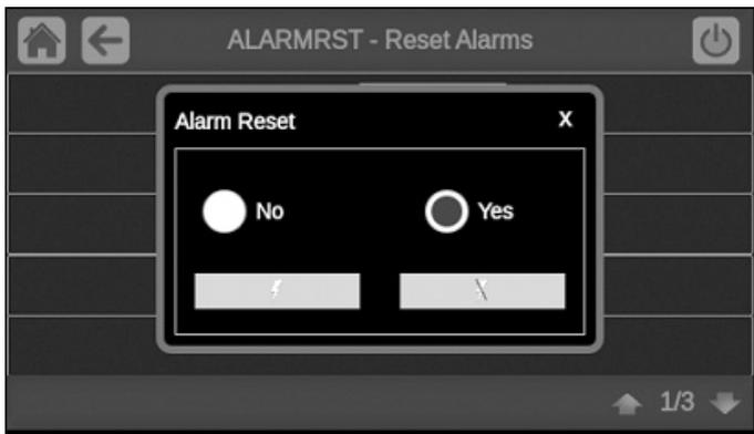
In the event of a power supply interrupt, the unit restarts automatically without the need for an external command. However, any faults active when the supply is interrupted are saved and may in certain cases prevent a circuit or a unit from restarting. Once the cause of the alarm has been identified and corrected, it will be displayed in the alarm history.
