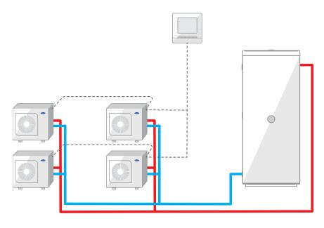
AquaSnap 30AWH-P can be cascaded with up to 4 units for heating and cooling requirements in light commercial applications.
