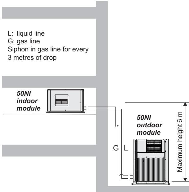
Note: when the unit is supplied for split version with the outdoor and indoor modules, can include optionally filling and service valves for the circuit connections and the charge of refrigerant until 7 m of distance.
