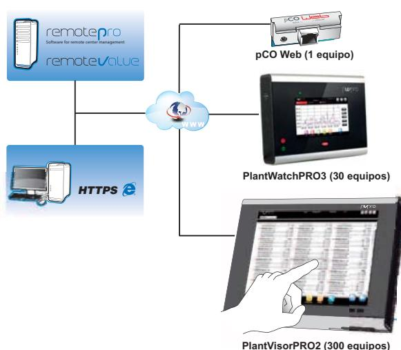
These systems allow the installation in remote management. Through a single connection to the Internet is accessed the information system. The Web interface, which is available for the local user, allows the monitoring and the complete configuration of the installation: from the office or any other user's current location.
