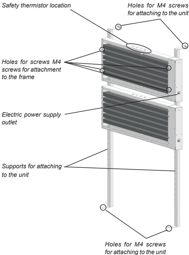
Step 2: attach the supports with the frames linked inside the unit. To that extent, drills have been made in the unit to which the supports must be screwed.
