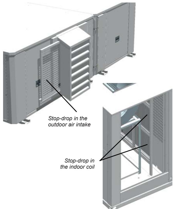
**Note:** with hot water coil (nominal or heater) it is not possible to assemble the stop-drop.
