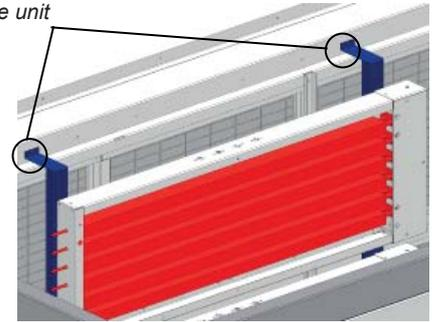
The supports attached to the unit can be seen in the following illustration.
