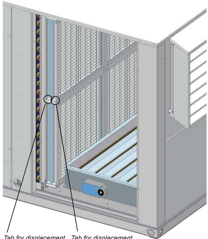
Tab for displacement of opacimetric filters
