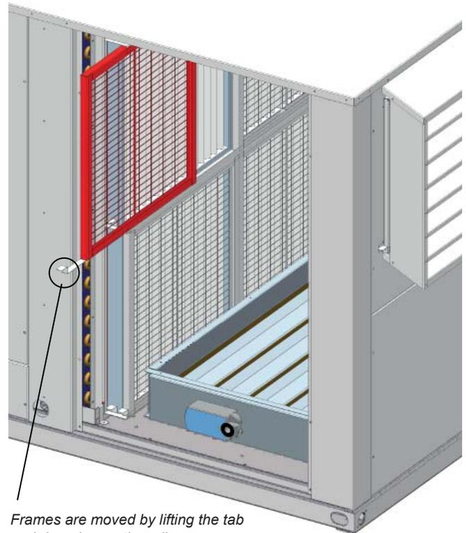
Frames are moved by lifting the tab and dragging on the rail
