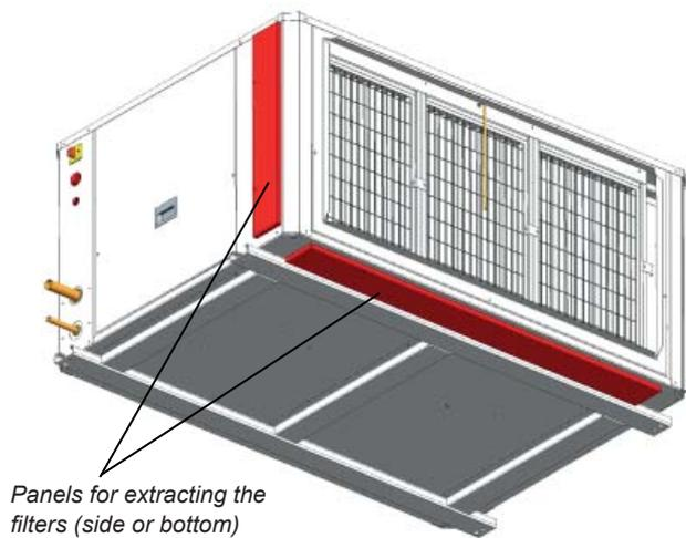
Panels for extracting the filters (side or bottom)
