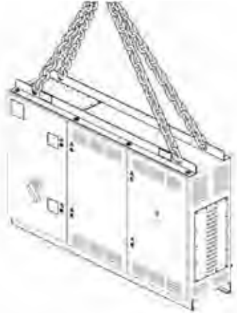
Fig. 54 - Lifting the VFD
