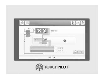
The bell located in the upper-right part of the screen lights when any fault is detected (see also section 8.2).
